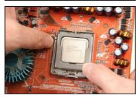
Place the heatsink and fan assembly onto the socket. Align the four fasteners toward the four mounting holes on the motherboard.
